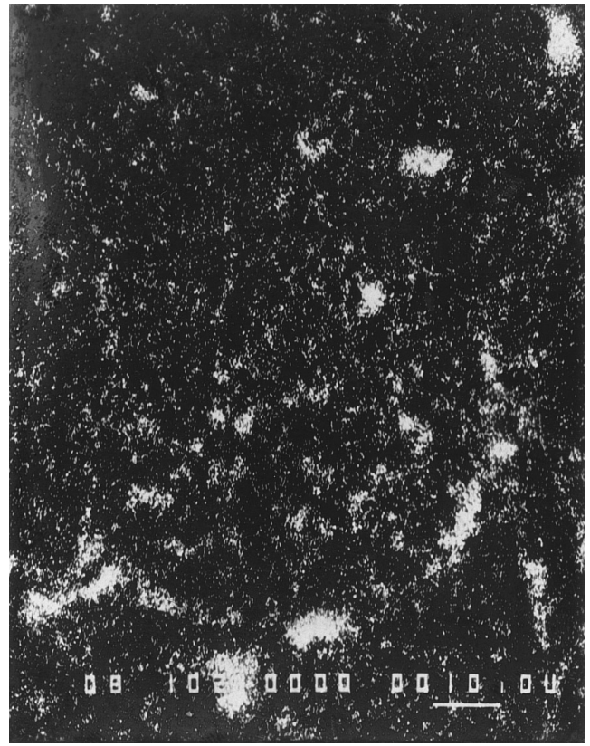
FIG. 4. SEM-EDS aluminum map of an aluminum (hydr)oxide coated Ottawa sand surface showing the regularly observed patchwise surface impurities (originally 680 \times magnification). Micrograph was representative of entire surface.
