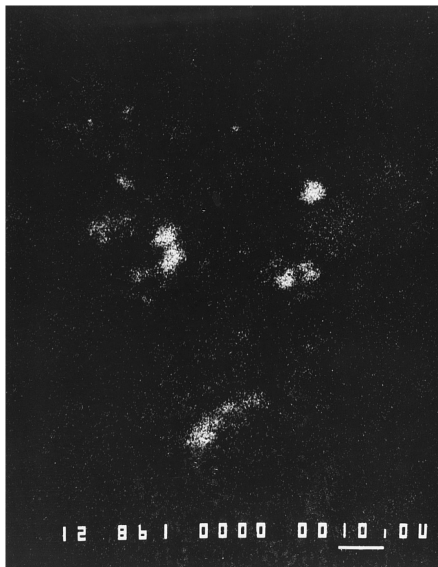
FIG. 2. SEMEM iron map of Ottawa sand surface showing a region of patchwise surface impurity, a source of the surface charge heterogeneity, and a site for potentially favorable particle interactions (originally 680× magnification). Occurrence of these iron sites was intermittently observed on the surface.
