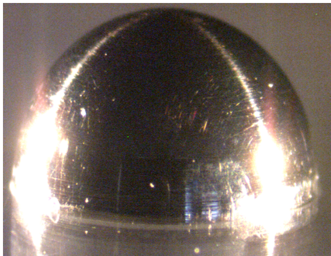
Figure 8-14: Side view of the hemispherical electrode after washing it with deionized water.
