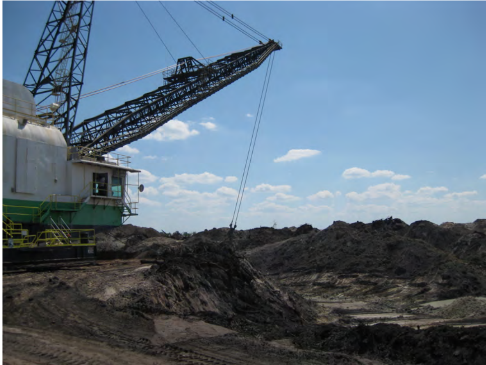
Figure 2-3. Photograph of electrically operated dragline shown mining the phosphate matrix (photograph by Mark Orazem, used with permission).
