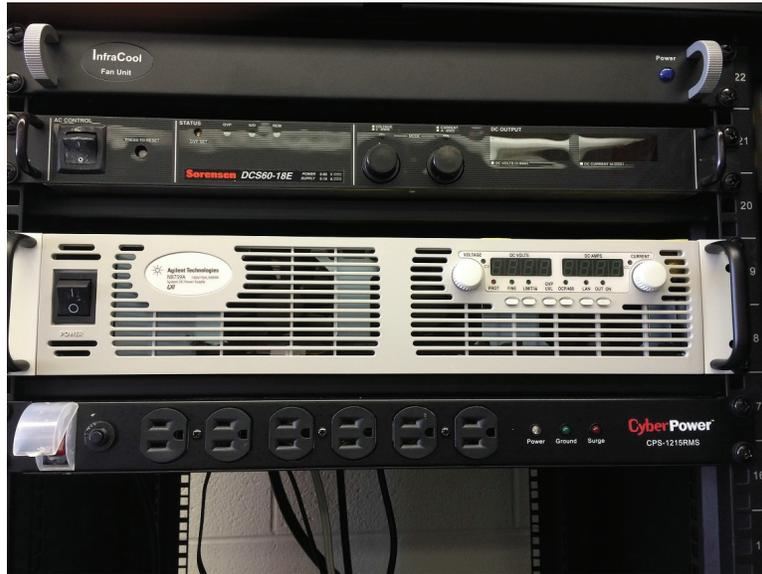
Figure 5-7. DC power supply of fully-continuous prototype (photograph by Rui Kong).
