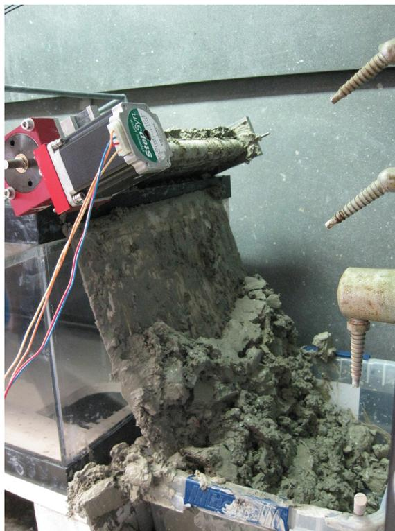
Figure 4-10. A container for thickened clay collection (photograph by Rui Kong).
