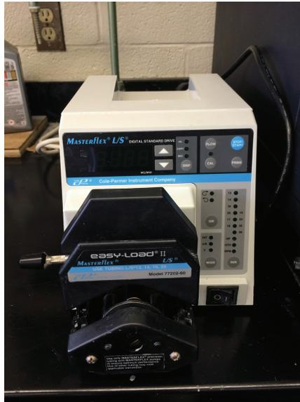
Figure 5-8. Water pump of fully-continuous prototype (photograph by Rui Kong).
