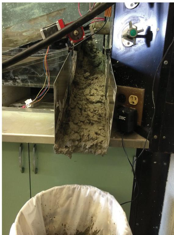
Figure 5-5. The collection tray of fully-continuous prototype (photograph by Rui Kong).
