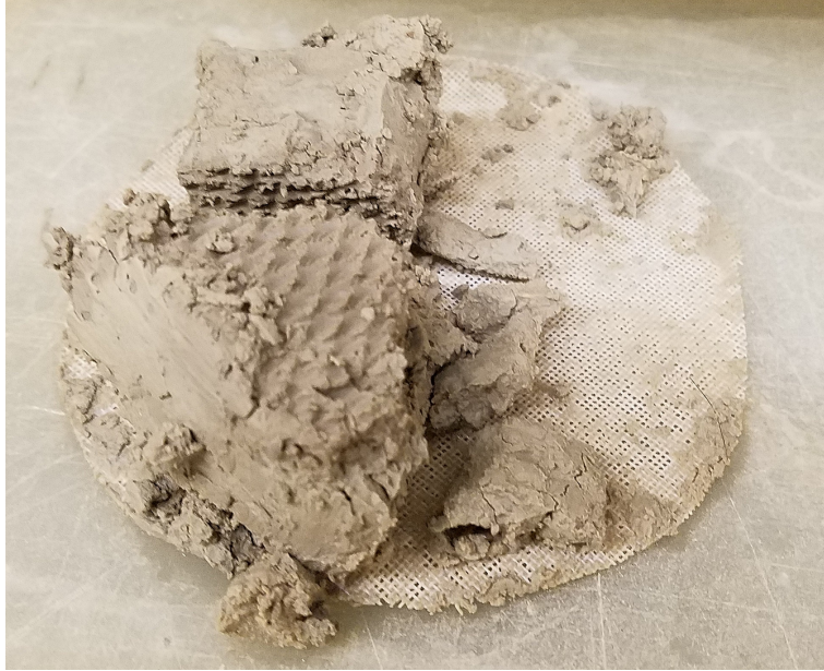
Figure 4-9. Clay cake with a solids content of 40 wt.% produced in the bench-top cell using a false-bottom cathode as the bottom electrode with constant electric field of 4 V/cm over 5 hours. Photograph courtesy of author.
