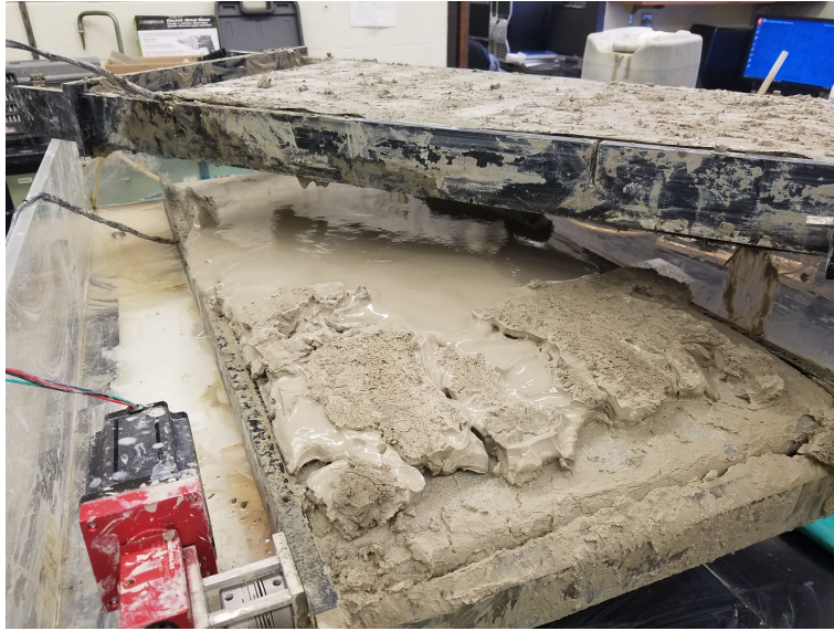
Figure 4-16. The dewatering unit was operated under the same conditions as in Figure 4-14. The fingers of low solids-content cake at the discharge was due to the clay sticking to the anode when the upper frame was removed. The progressive dewatering as the clay travels down the unit is observed. Photograph courtesy of author.
