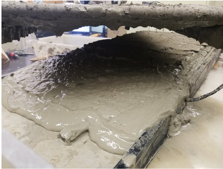
Figure 4-10. Dewatering unit from the feed side without the top frame. The feed-side electric field was 2.1 V/cm and the belt speed was 0.38 cm/min. The unit was fed sludge with a solids content of 13 wt.%. This image was taken from an experiment used to troubleshoot the prototype and was not used in the economic analysis. Photograph courtesy of author.
