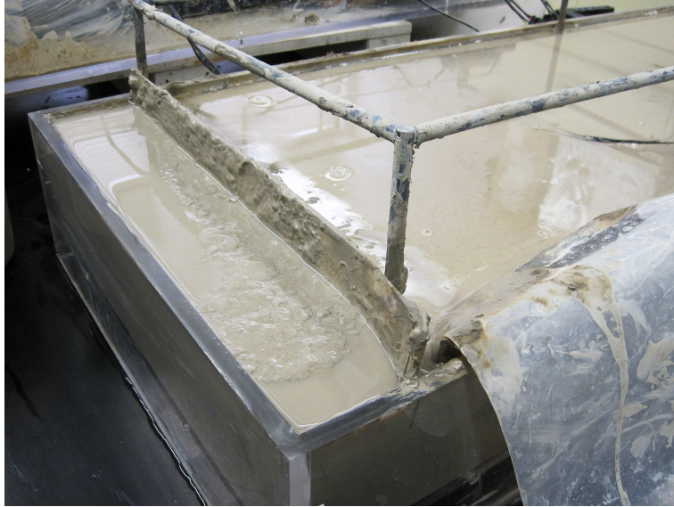
Figure 4-4. Collection area of the clay thickening unit after batch-wise collection of the thickened sludge. The sludge production continued at the same operating parameters as stated in Figure 4-3 until a sufficient amount accumulated prompting the next collection. Photograph courtesy of author.
