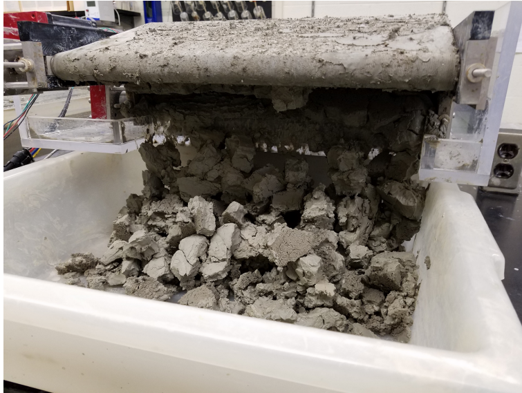
Figure 4-12. Collected clay cake collected at the discharge of the dewatering unit in the two-stage design. The photograph was taken on the same experimental run as the images shown in Figures 4-10 and 4-11. The unit produced cake with a solids content of 36 wt.% at 3.2 kg/hr which corresponds to a dry-clay production rate of 1.2 kg/hr. This image was taken from an experiment used to troubleshoot the prototype and was not used in the economic analysis. Photograph courtesy of author.
