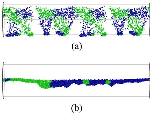
FIG. 4 (color online). Snapshots of the particle distribution generated by an oscillating gravitational field,  $g = g_0 \times \sin(\pi u_s t/R)$  in the vertical direction; (a) including the flow field generated by the no-slip boundary condition on the cylinder wall, and (b) excluding the flow field generated by the no-slip boundary condition on the cylinder wall. The green (lighter) particles are moving to the right, while the blue (darker) particles are moving to the left.
