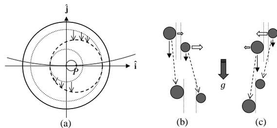
FIG. 2: (a) Single particle trajectory neglecting centrifugal migration. (b, c) Relative velocity of two particles sedimenting with different settling velocities: (b) when the particle behind falls faster than the particle in front, they repel each other; (c) when the particle in front falls faster, they attract.
