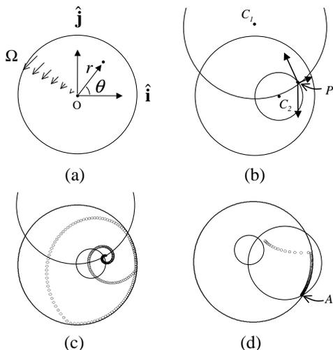
FIG. 1: Characterization of isolated particle dynamics: (a) the coordinate system used in Eq. 1; (b) Circles  $C_1$  and  $C_2$  describe the locus of points of zero radial and angular velocity; (c) spiral motion of a single particle placed near the unstable equilibrium point,  $P$ ; (d) when  $D_2 > 1$ , a particle cannot have closed trajectory.
